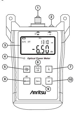
Figure 1 CMA5 Series Power Meter Operating Controls
