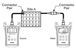
Figure 3 Patch Panel to Connecto
